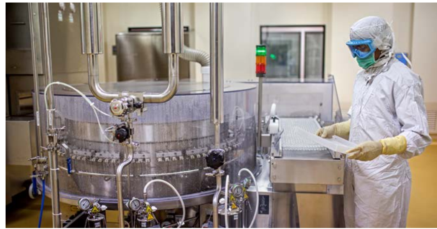
Pentavalent vials are being washed and sterilized before being filled with vaccine. The pentavalent vaccine is a single vaccine that protects against five major childhood diseases: hepatitis B, Haemophilus influenzae type b, diphtheria, tetanus and pertussis
